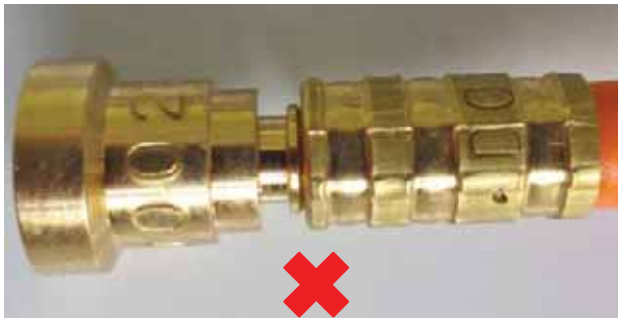
Insert not crimped in the proper position
