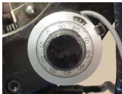
Electro Mechanical control with vernier dial
