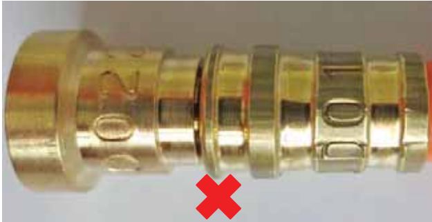
Example of ferrule not completely swaged
