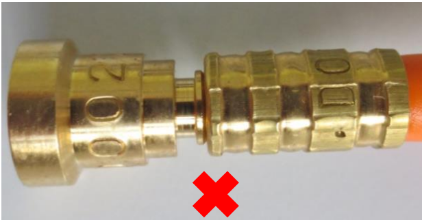
Insert not crimped in the proper position
