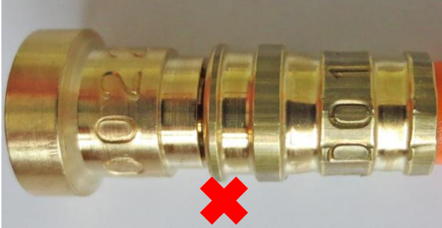
Example of ferrule not completely swaged
