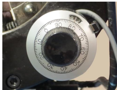
Electro Mechanical control with vernier dial
